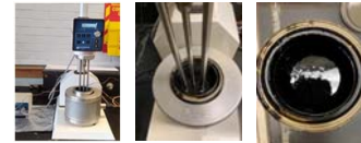
High shear mixer, 30 minutes, 165°C
